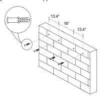
2. Install 4 dry wall anchors on the wall.
