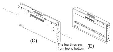
**STEP C.** Take off the screws (The fourth screw from top to bottom) in both sides of fireplace. **Figure (C)**
