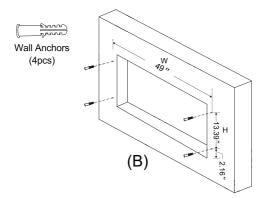
$\mbox{\bf STEP B}.$  Punch 4 holes around the wall and install 4 Drywall anchors (Part C) , please drive C completely into the wall.
