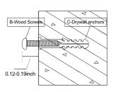
3. Install 4 wood screws, taking care not to screw them in completely. Screw head exposed 0.12-0.19inch distance.
