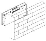
4. Two people lift the fireplace and hang the 4 clipson the back on the 4 dry wall anchors.
