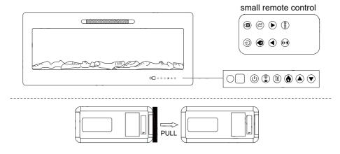
Remove the romote control insulation sheet.
