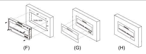
STEP F. Take off the two screws in both sides of fireplace. Figure (C) If the appliance is fully recessed into the wall:
