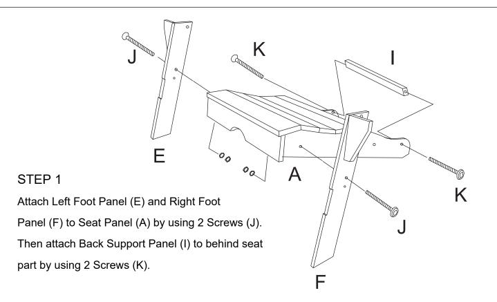
Note: Do not tighten all screws until last step.
