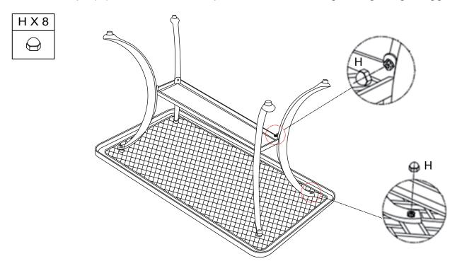
Step 4 Stand the table right side up. Adjust the Legs pre-installed Levellers until the Table is level with the ground.
