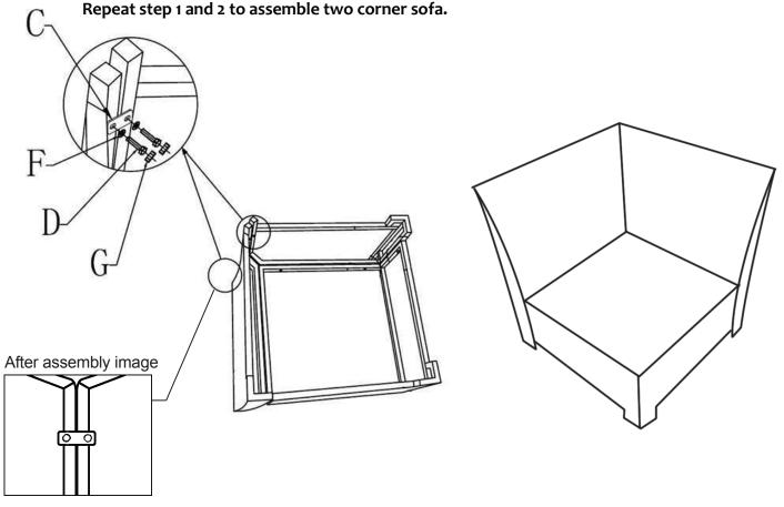
Step 3 Atach back panel A1 to seat panel B2 by using 4 long Bolts (E) and 4 Washers (F). Finally put bolt Caps (G) untl all parts have been connected and bolts are tightened. Repeat to assemble two armless sofa.
