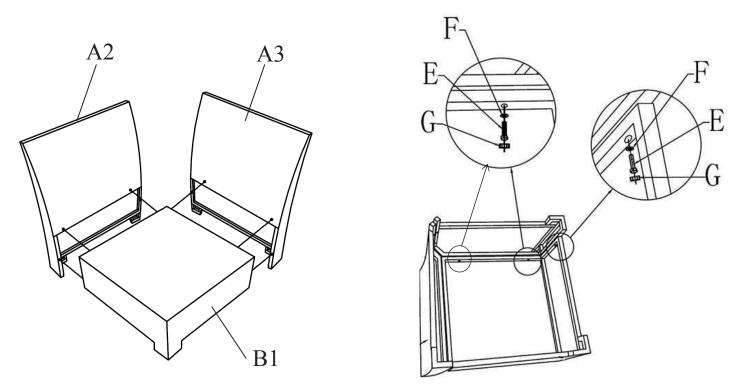
Step 2 Connect the two back panels by using 2 Connectors (C), 4 short Bolts (D) and 4 Washers (F). Finally put bolt Caps (G) untl all parts have been connected and bolts are tightened.
