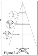
Step 3 Unfold the branches one-by-one beginning with the lowest.
