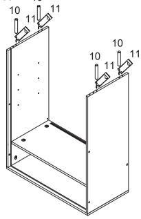
STEP 11 Slide back panel (L) into the grooves of left wood panel (F) and right wood panel (G). Place
