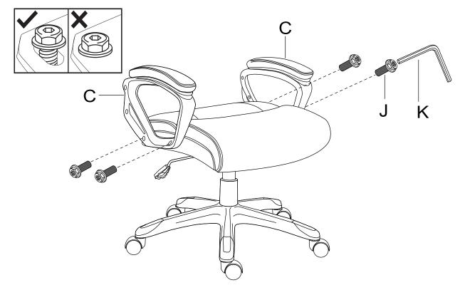
Attach the Back (A) to the Armrest (C) by using Allen Bolt (J) and Allen Wrench(K). Ensure all the Bolts are tight with Allen Wrench.
