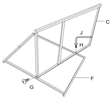
Attached the Left Side Frame (E) to the Back Frame (C) by using Allen Bolt (G), Allen Bolt (H) and Allen Wrench (J) as shown in below diagram.
