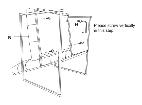
STEP 6 Please 100% tighten all bolts and screws completely until the entire unit has been assembled and set up. After initial assembly, the product may acclimate to its new environment. Please ensure all screws are still securely tightened.
