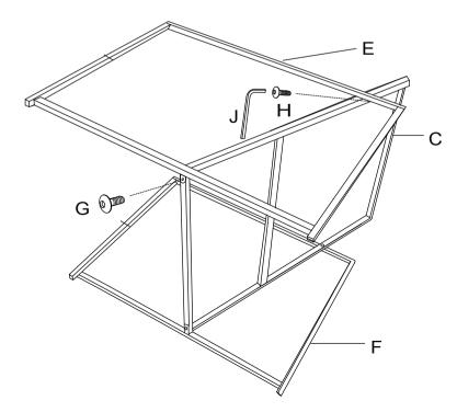
Attached the Seat Frame (D) to the Back Frame (C) and Side Frames (E&F) by STEP 3 using Allen Bolt (G), Allen Bolt (H) and Allen Wrench (J) as shown in below diagram. Please 80% tighten the bolts.
