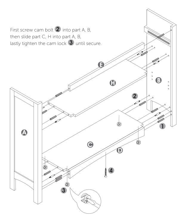
Push cam lock into the hole, then take a flathead screwdriver (as pictured) and twist 45 degrees until it is locked in place.
