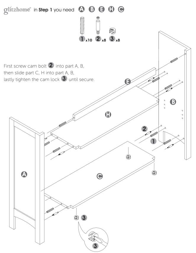
Push cam lock into the hole, then take a flathead screwdriver (as pictured) and twist 45 degrees until it is locked in place.
